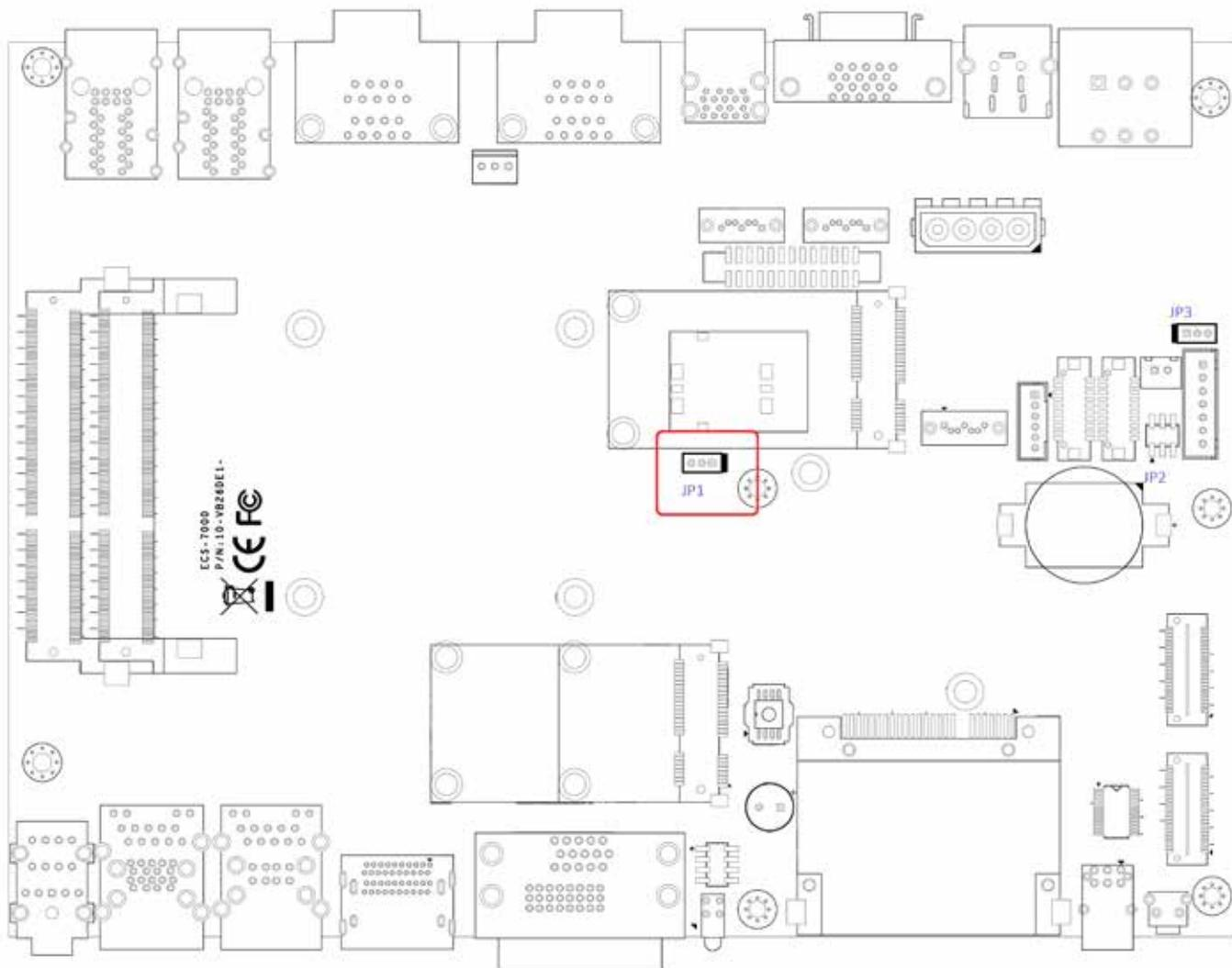
The ECS-7000 main board contains a jumper that can switch the AT/ATX Power Setting. Normally this jumper should be set with Pin 4 and Pin 6 in ATX power mode. And power on the system by the 2-pin terminal block at the top panel. If you set it with Pin 2 and Pin 4 in AT power mode. It will send the power button signal to power on the system automatically
