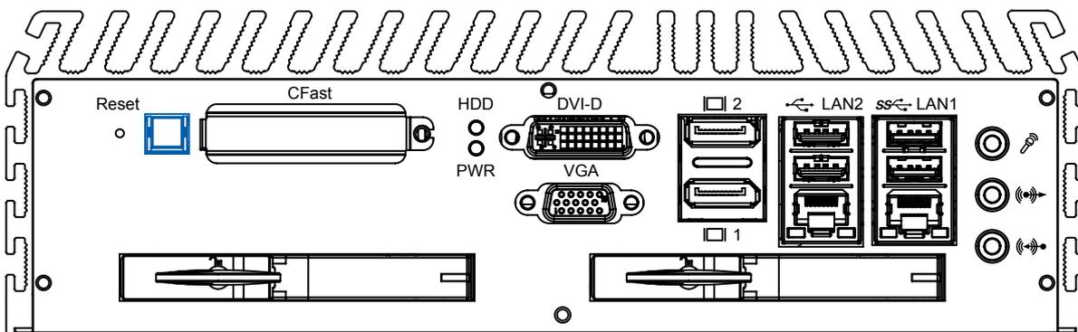
The power button is a non-latched switch with dual color LED (Blue/Orange) for indication S0, S3 and S5 status. Power button dual-color LED indicator:
