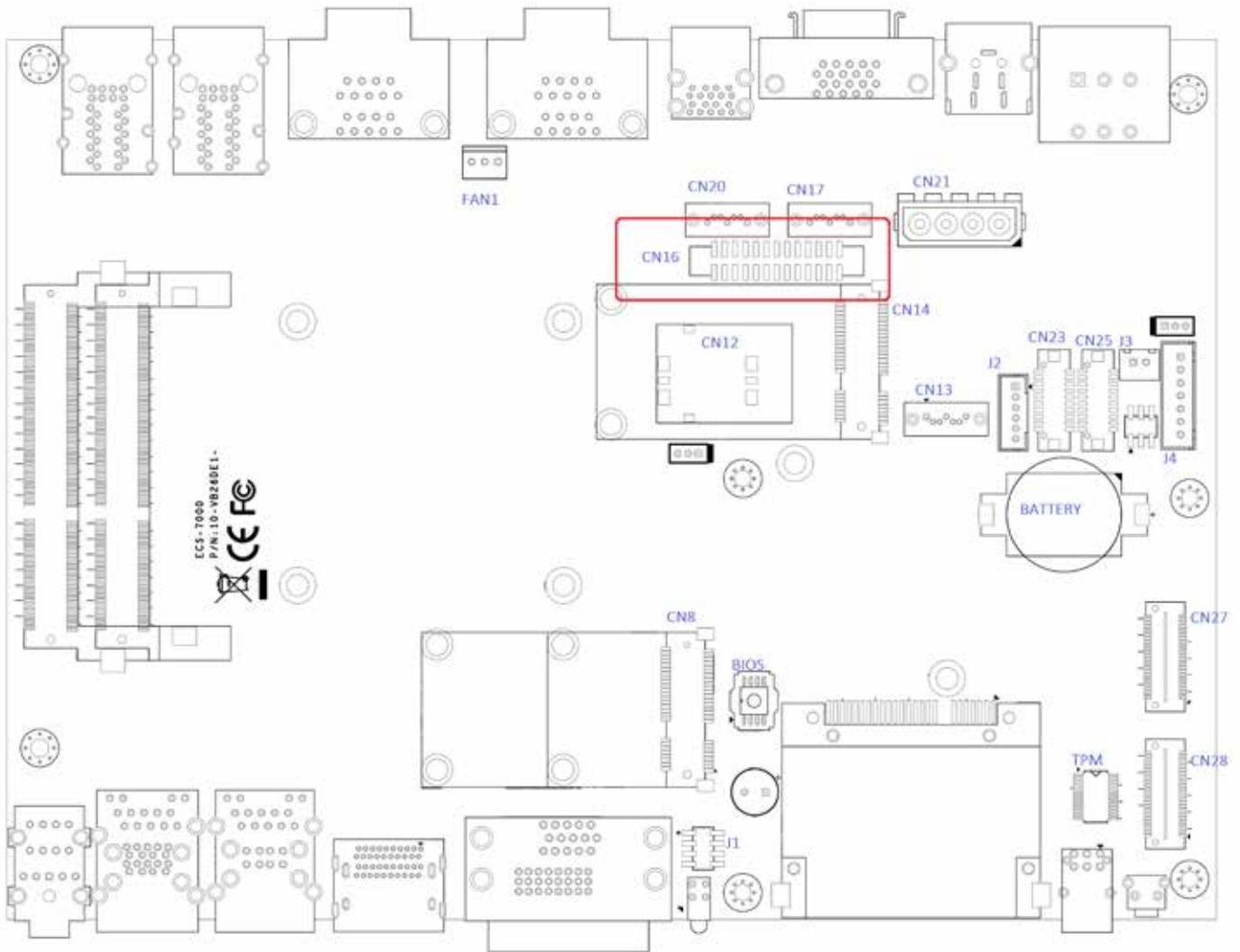
The ECS-7000 series offers 16 programmable I/O within TTL 5V tolerance. If the GPIO is logic high, it indicates that the mapping SIO GPIO pin is logic high level. If the GPIO is logic low, it indicates that the mapping SIO GPIO pin is logic low level.
