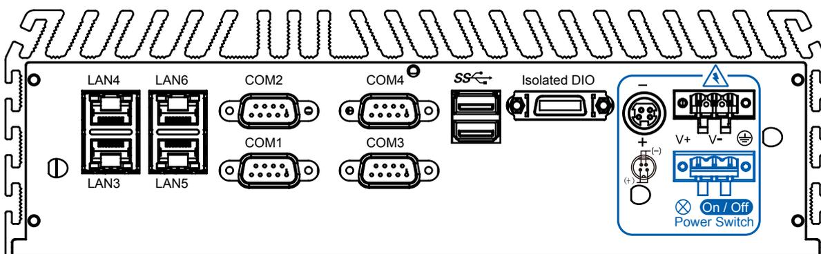
It is a 2-pin power-on or power-off switch through Phoenix Contact terminal block. You could turn on or off the system power by using this contact. This terminal block support dual function of soft power-on / power-off (instant off or delay 4 second), and suspend mode.
