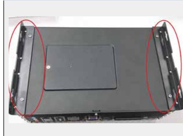
Fix two wall-mount brackets to the chassis with four M4 screws using a Philips screwdriver.
