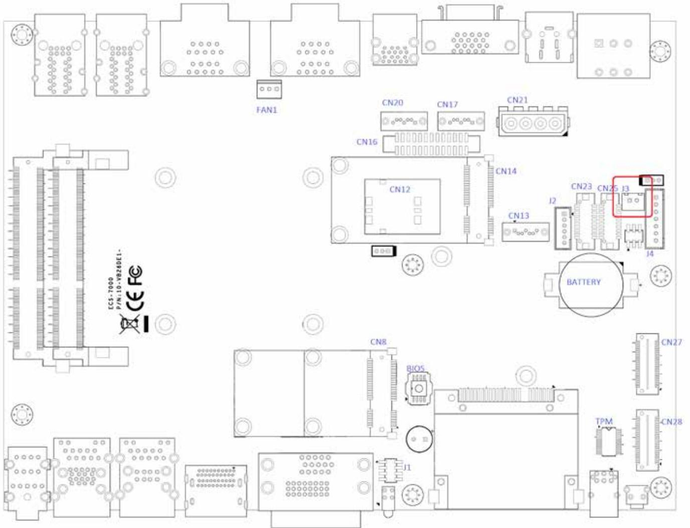
The ECS-7000 series is also equipped one SATA DOM power connector. It supplies 5V (0.5A max.) current to the SATA DOM.
