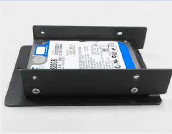
Place the HDD into the bracket and gently push it down to make it contact with thermal pad. Use a Philips screwdriver to fix the HDD with M3 screws. Please note that the HDD must be placed in the right direction as below.
