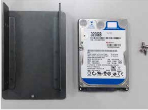
Find the HDD bracket come with "Pet-Door", M3 screws (4 pieces), and HDD thermal pad (1 piece) in the accessory box.
