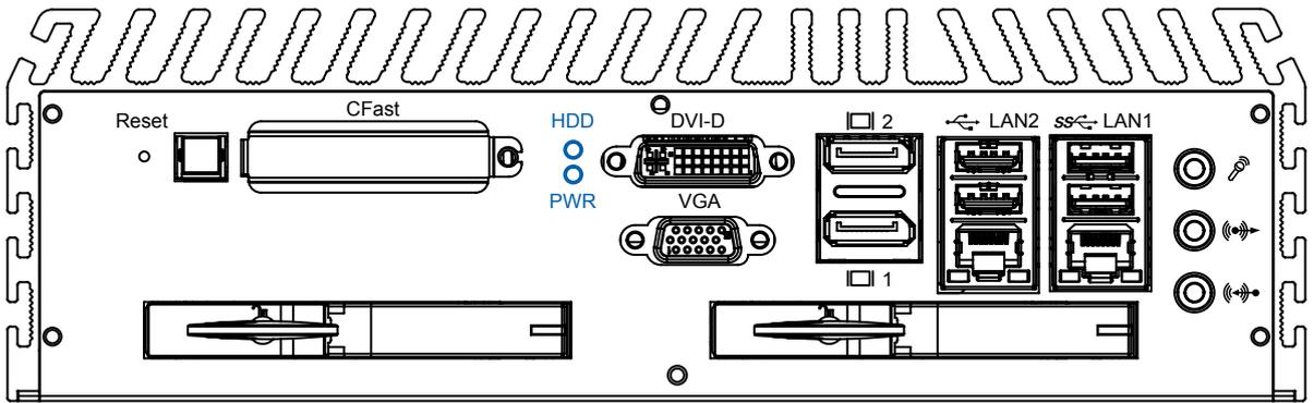
Yellow-HDD LED: A hard disk / CFast LED. If the LED is on, it indicates that the system's storage is functional. If it is off, it indicates that the system's storage is not functional. If it is flashing, it indicates data access activities.
