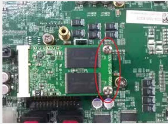
Using 2 BH-M2.5X6 screws to lock your mini-PCIe card firmly. Then you can re-screw the back panel as the first step.
