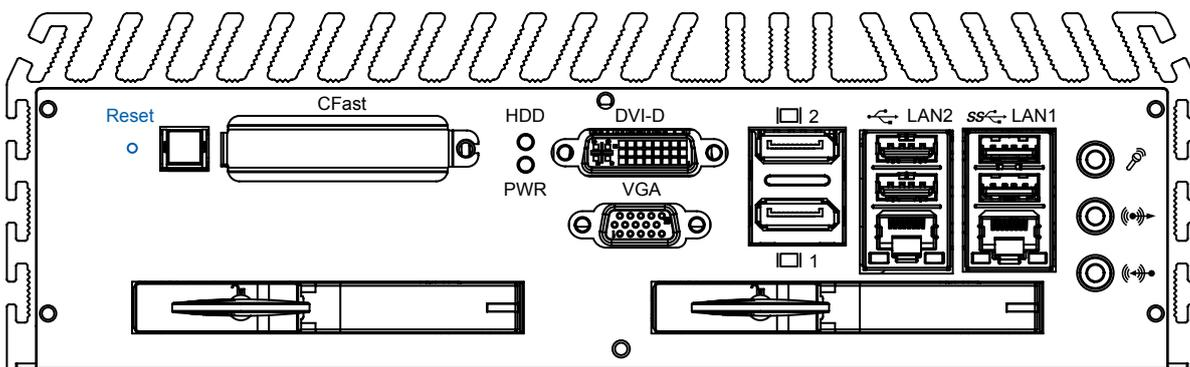
It is a hardware reset switch. Use this switch to reset the system without turning off the power. Momentarily pressing the switch will activate a reset.
