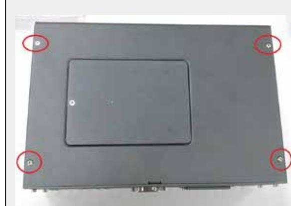
Put the ECS-7000 series upside down on a flat surface. Use a Philips screwdriver to loose screw on the back side.
