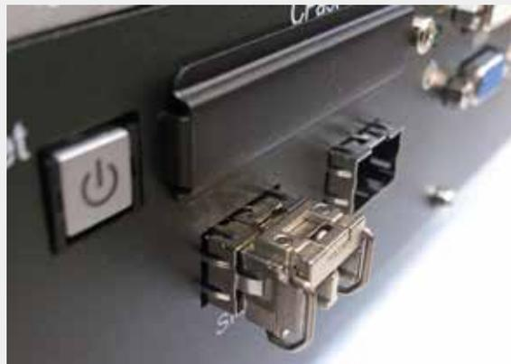
Pushing the Fiber module to the socket till it locked to the socket firmly. Repeat Step 2 if you are inserting a second SFP module. Do not remove the SFP module plugs until you are ready to install the cables.
