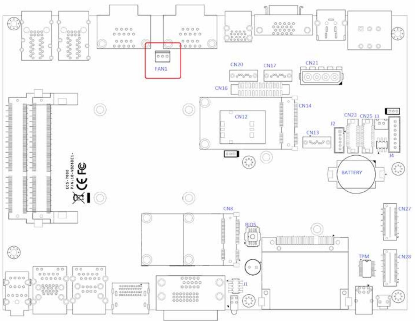
FAN power connector supports for higher thermal requirement.
