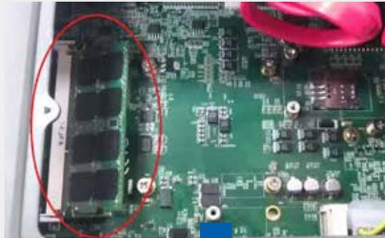
Tile the SODIMM module and insert it to the SODIMM socket.
