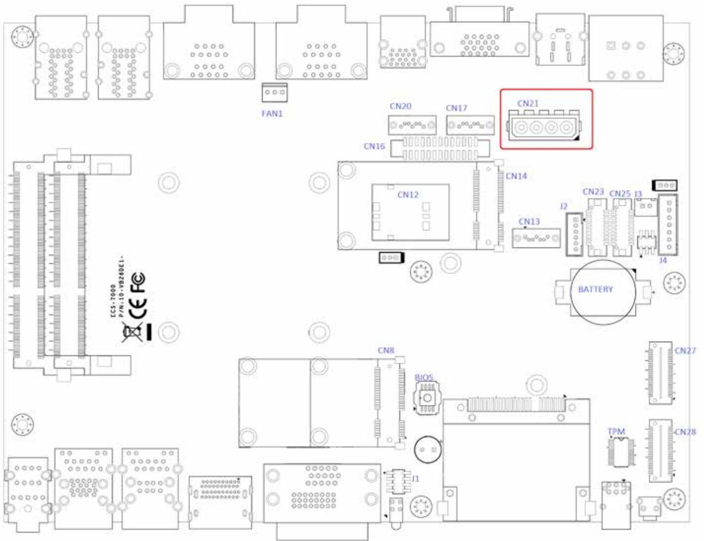
The ECS-7000 series is also equipped one SATA power connector. It supplies 5V (2A max.) and 12V (1A max) current to the hard drive or SSD.
