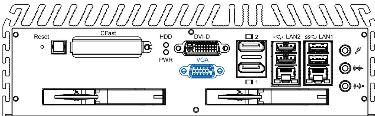
The ECS-7000 series comes with a DB15 female connector on the front panel to connect a VGA monitor. To ensure that the monitor image remains clear, be sure to tighten the monitor cable after connecting it to the ECS-7000 series. The VGA output mode supports up to 1920x1200 resolutions. The pin assignments of the VGA connector are shown below.
