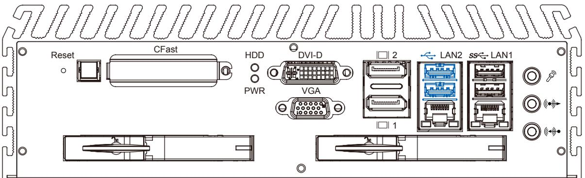
The ECS-7000 series comes with 2 USB 2.0 hosts on the front panel. The USB interface supports Plug and Play, which enables you to connect or disconnect a device whenever you want, without turning off the system. The hosts can be used for an external flash disk or hard drive for storing large amounts of data. You can also use these USB hosts to connect to a keyboard or a mouse. The following diagram shows the pinouts for USB1 and USB2 port.
