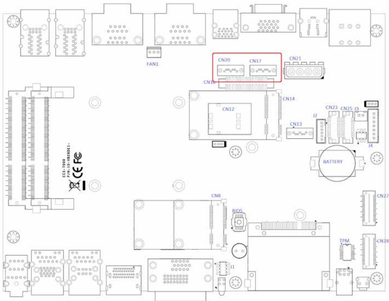
The ECS-7000 series features 2 high performance Serial ATA III interfaces that ease cabling to hard drives or SSD with thin and short cables while application need larger storage capacity.
