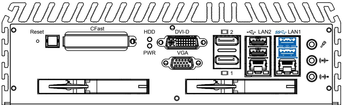
The ECS-7000 series comes with 2 USB 3.0 hosts on the front panel. These USB 3.0 ports allow data transfers up to 5 Gb/s. The controller supports SuperSpeed (SS), high-speed (HS), full-speed (FS) and low-speed (LS) traffic on the bus.
