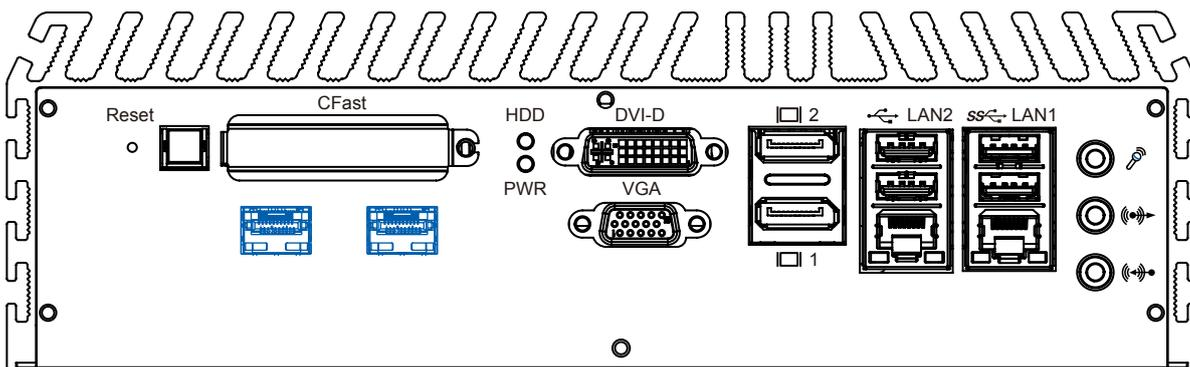
The SFP modules are input/output devices that plug into a Gigabit Ethernet (GE) port, linking the port with a 1000BASE-X fiber-optic network.
