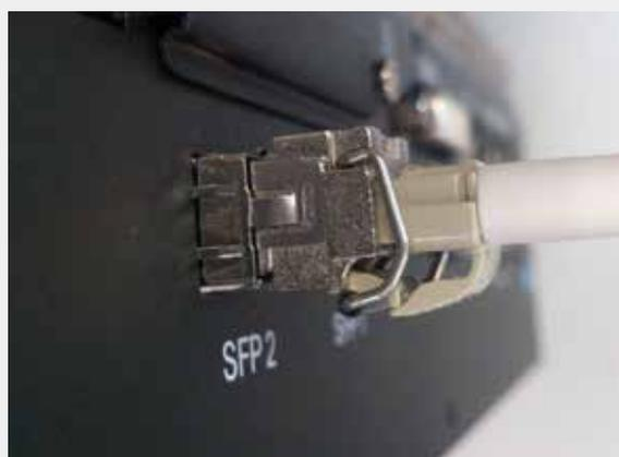
Loose the swing latch to unlock the Fiber Module and SC cable connection.
