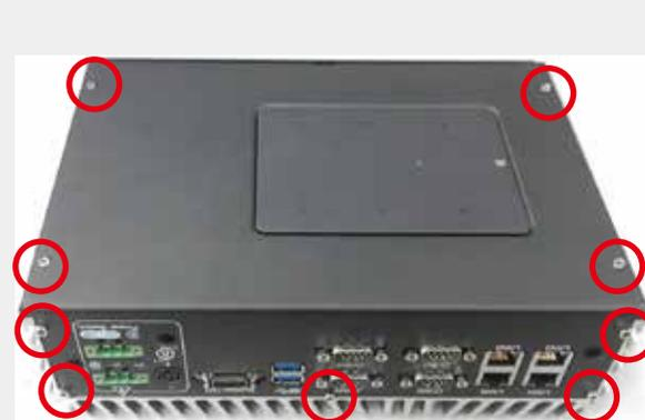
Use a screwdriver to loose 9 screws on the "Back Panel". Find the BH-M2.5X6 (4 pieces) screws pack in the accessory box.
