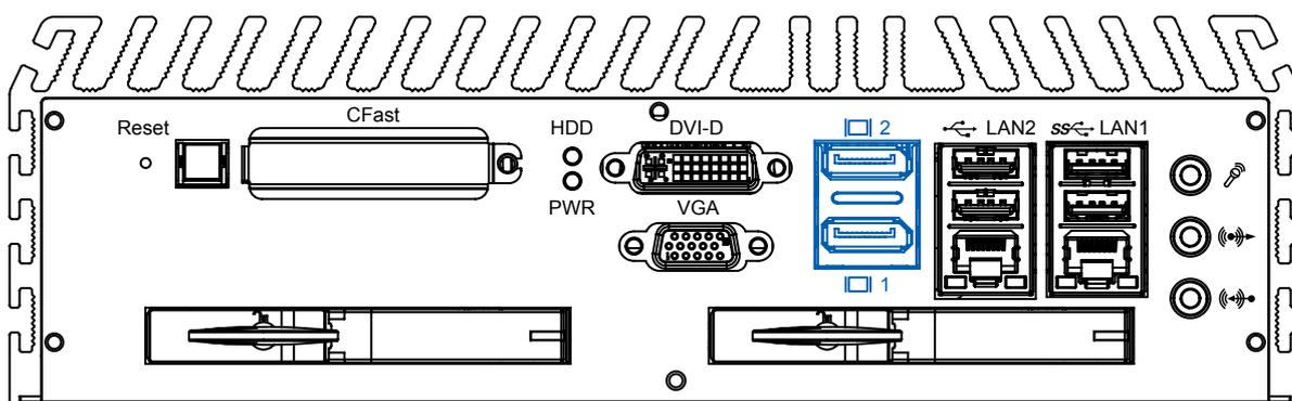
Each digital port is capable of driving resolutions up to 2560x1600 at 60 Hz through Display Port.
