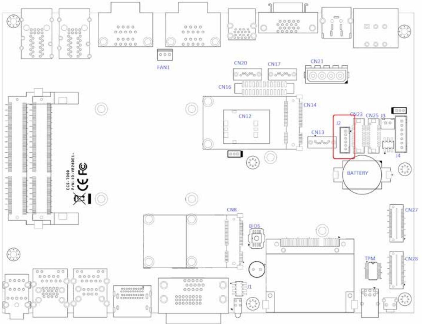
The ECS-7000 series' main board provides up to two USB plug-and-play ports for Dongle Key or LCD touch Panel using. The USB interface supports 480 Mbps transfer rate which complies with high speed USB specification Rev. 2.0, and fuse protection. The USB interface is accessed through one 1x6-pin JST 2.0mm connector. You will need an adapter cable if you use a standard USB connector. The adapter cable has a 1x6-pin connector on one end and a USB connector on the other.
