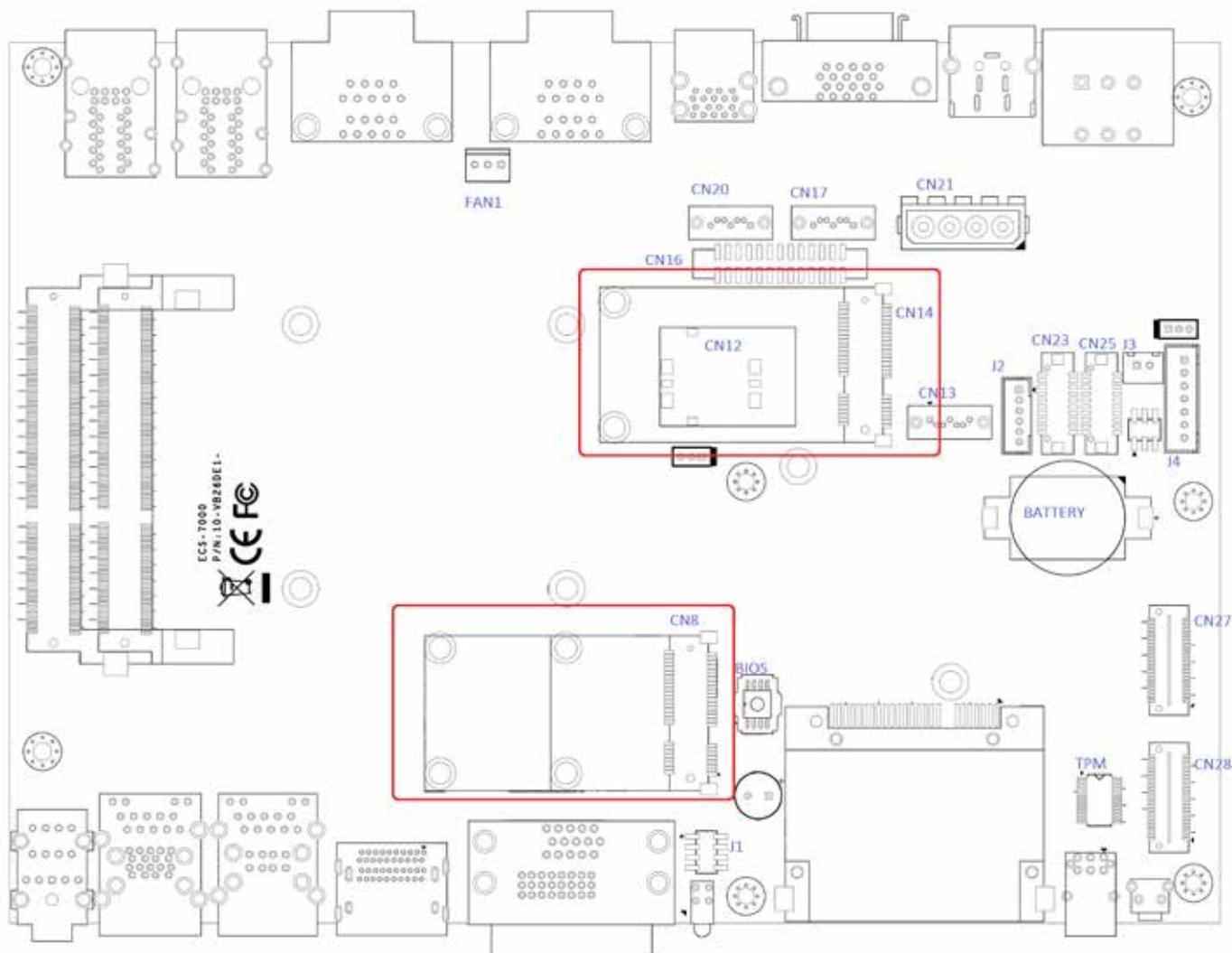
Both mSATA and Mini PCI-E share the same form-factor and similar electrical pinout assignments on their connectors. There was no clear mechanism to distinguish if a mSATA drive or a Mini PCI-E device is plugged into the socket until recently that SATA-IO issued an ECN change (ECN #045) to re-define pin 43 on mSATA connector as “no connect” instead of “return current path” ( or GND).
