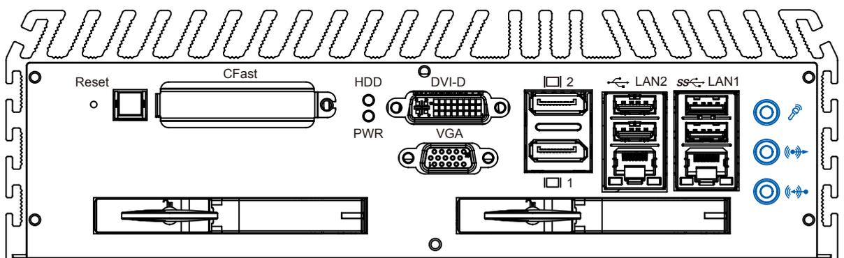
The ECS-7000 series offers stereo audio connector of MIC , Line\_In and Line\_Out. The audio chip controller is by ALC892 which is compliant with the Intel® Azalia standard. To utilize the audio function in Windows, you need to install corresponding drivers for both Intel QM77 chipset and Realtek ALC892 codec. Please refer to Section 4 for information of driver installation.
