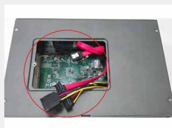
Remove the "Pet-Door" and you can see a SATA cable and DDR3 SODIMM socket exposed.
