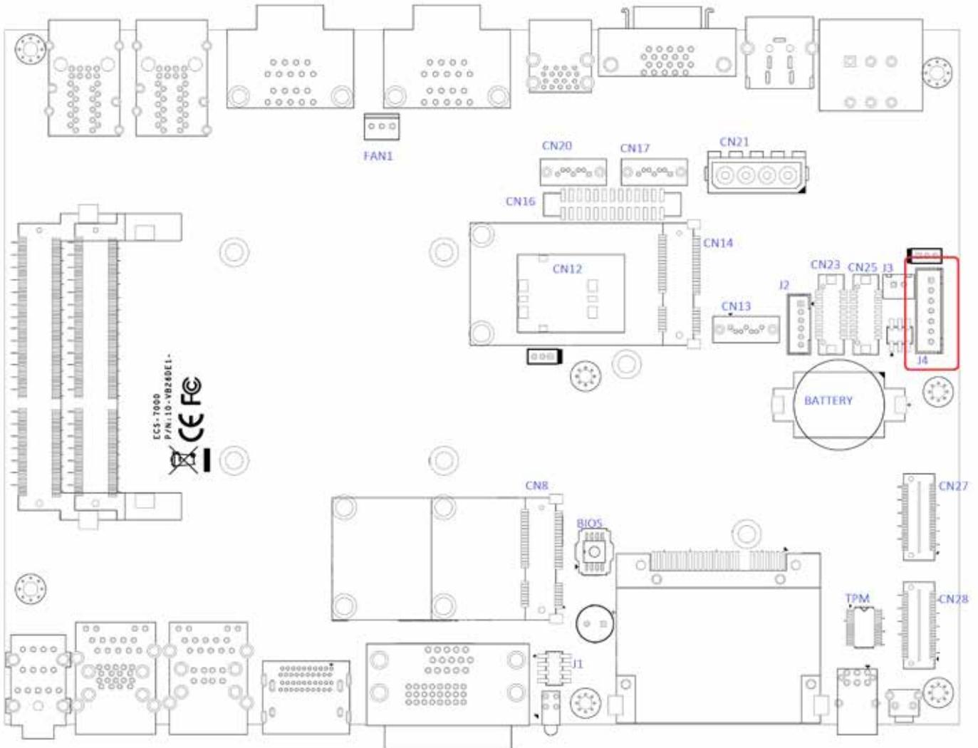
The LCD inverter is connected to J4 via a JST 7-pin, 2.5mm connector to provide +5V/+12V power to the LCD display.
