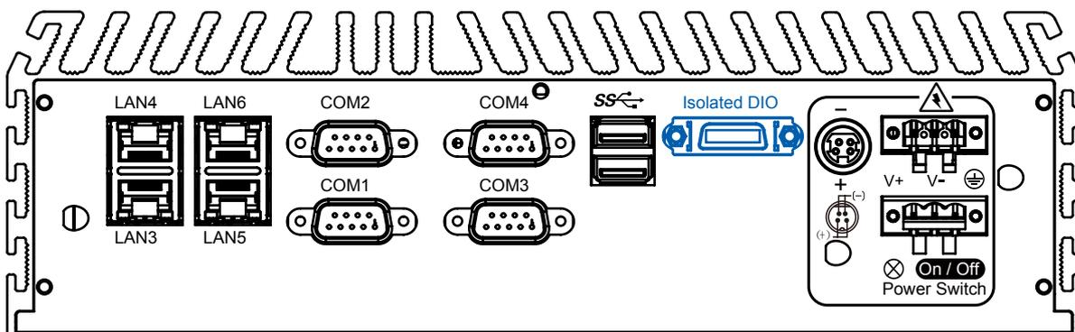
The ECS-7000 series offers an 16-bit DIO ( 8-DI / 8-DO) connector. Each bit of DI and DO equipped with a photo-coupler for isolated protection. A power buffer device TPD2007F integrated in 8-DO circuit for motors, solenoids, and lamp drivers applications.
