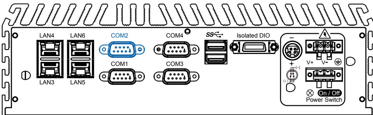
Serial port 2 can be configured for RS-232, RS-422, or RS-485 with auto flow control communication. Serial Port 2 default setting is RS-232, if you want to use RS-422 or RS-485, you can find the setting in BIOS.
