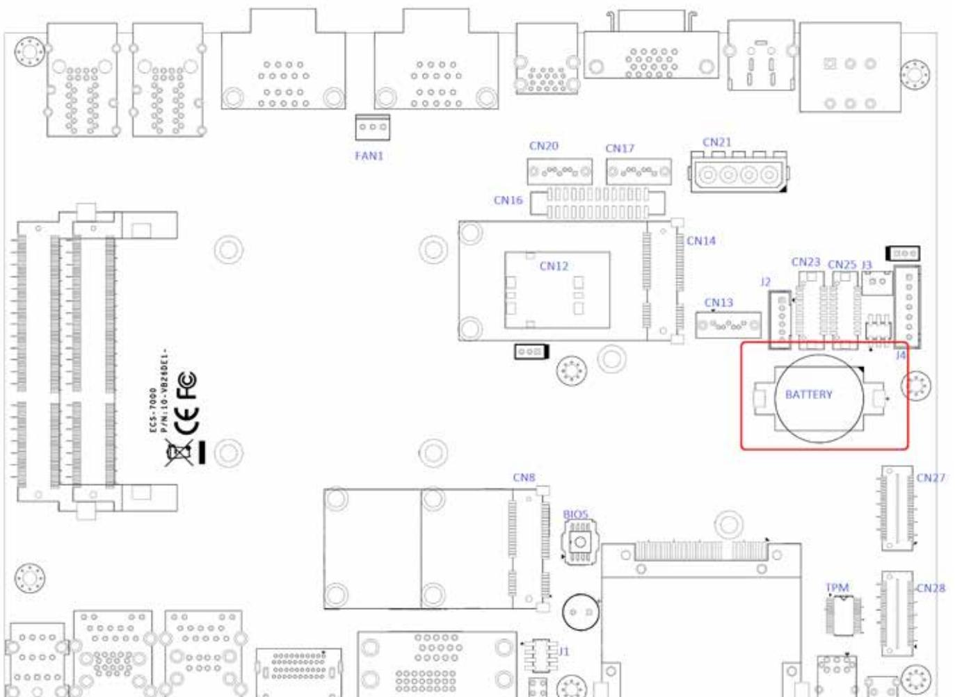
The ECS-7000 series' real-time clock is powered by a lithium battery. The battery is Panasonic BR2032 190mAh lithium battery. Replacing the lithium battery on your own is **NOT** recommended. If the battery needs to be changed, please contact with the Vecow RMA service team.
