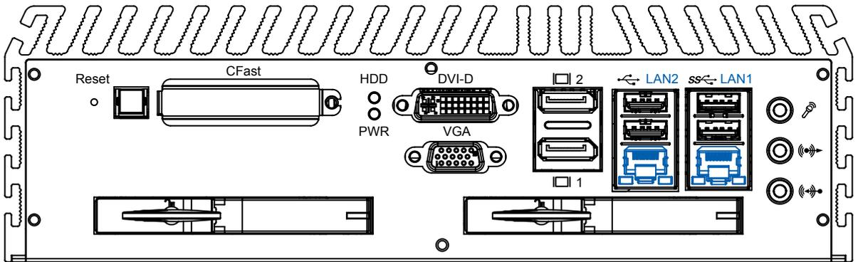
The 10/100/1000 Mbps Ethernet LAN ports 1 and 2 use 8-pin RJ-45 connector. LAN1 is equipped with Intel 82579LM for AMT function. LAN2 is equipped with Intel 82574L. Using suitable RJ-45 cable, you can connect ECS-7000 series system to a computer, or to any other piece of equipment that has an Ethernet connection, for example, a hub or a switch. Moreover, both of them have Wake-on-LAN and Preboot Execution Environment capabilities. The following diagram shows the pinouts for LAN1 and LAN2 port.
