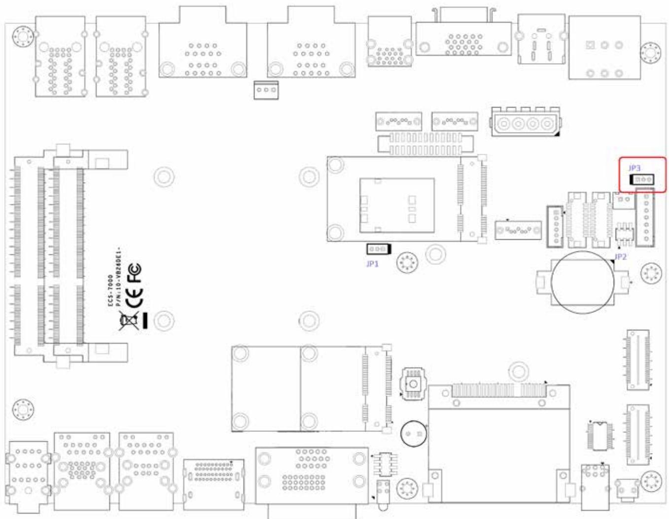
JP1 provides LVDS voltage selection function, closing Pin 1, 2 is for 3.3V LVDS power input; closing Pin 2, 3 is for 5V LVDS power input.
