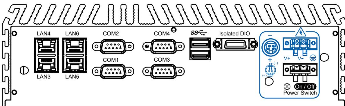
The ECS-7000 series offers 6 to 36 VDC power input with the terminal block. If the power is supplied properly, the Power LED will light up a solid green.
