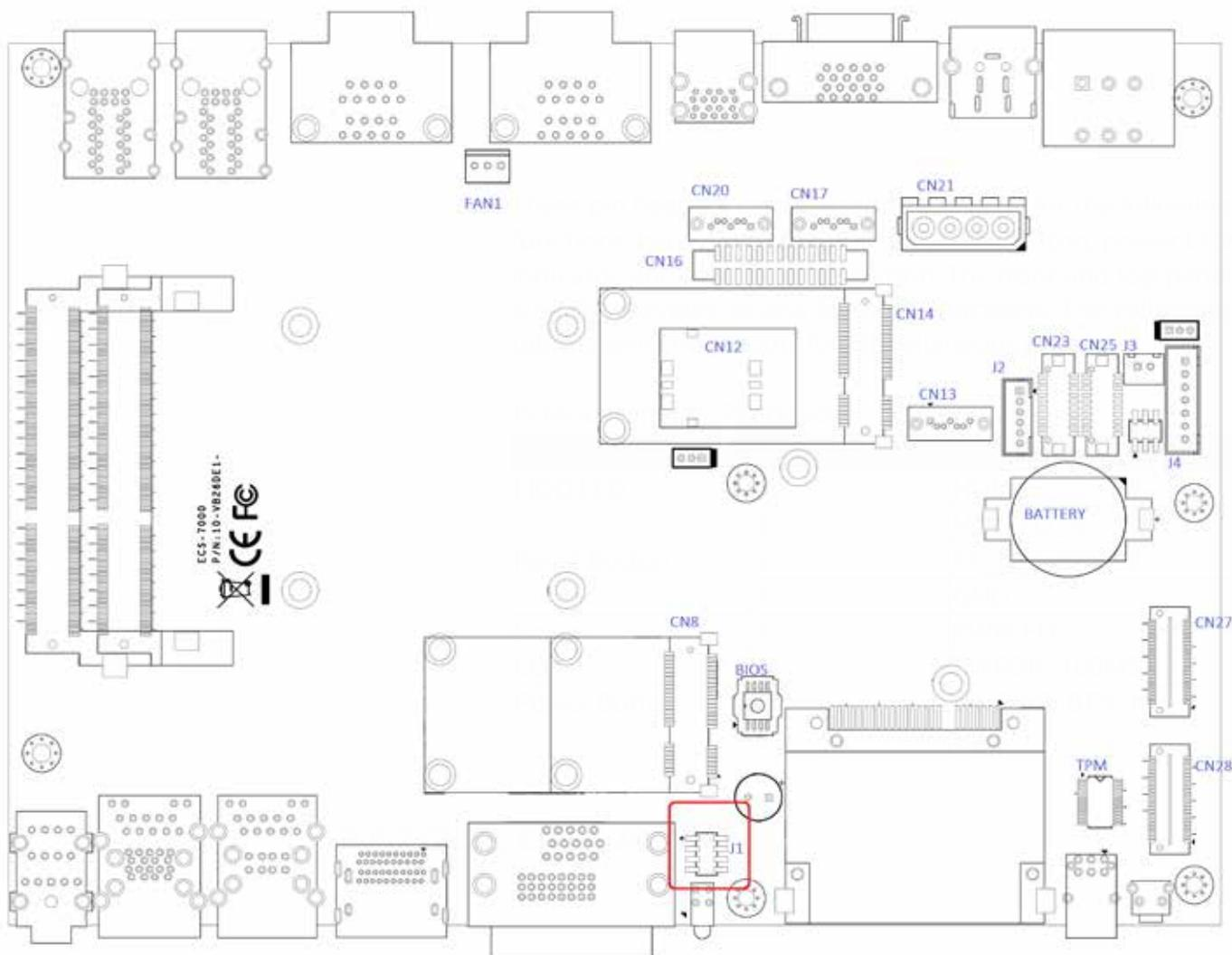
These pin headers can be used as a backup for the following functions: hard drive LED indicator, reset button, power LED indicator, and power-on/off button. The front and top panel already provides access to these functions. The following table shows the pinouts for Miscellaneous port:
