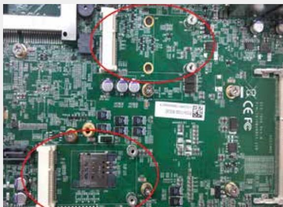
There are 2 Mini-PCle sockets on the main board. Choose one of Mini-PCle socket to put your mini-PCle card in.
