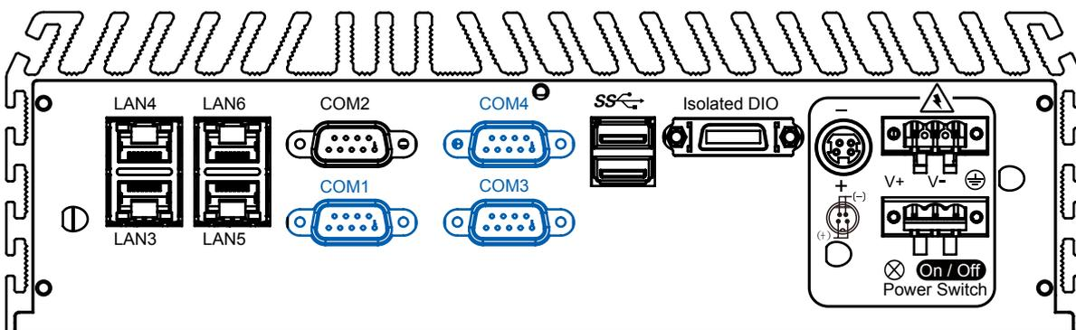
COM1, COM3 and COM4 are RS-232 only and provide up to 115200 bps baud rates. The pin assignments are shown in the following table:
